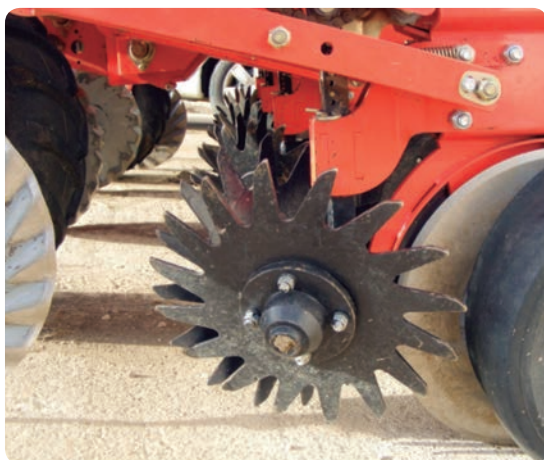
Fig. 3.16. Stubble sweeper mounted on the sowing train.
