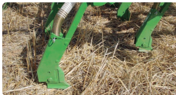
Fig. 3.20. Seed drill equipped with tines.
