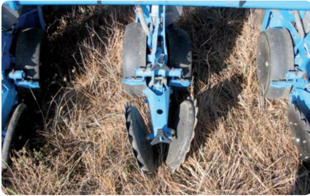
Fig. 3.21. Detail of row closure using double disc.
