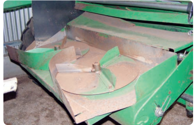
Fig. 3.22. Detailed system spreader of residues in the cereal harvester.
