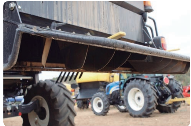
Fig. 3.23. Rear crop residue spreader detail.
