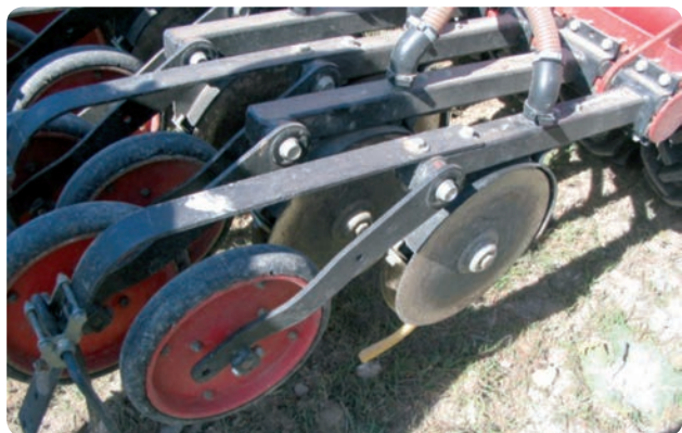
Fig. 3.18. Seed drill equipped with double disc opener.
